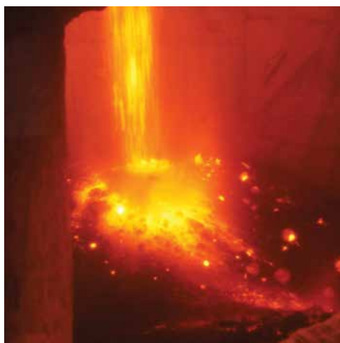
Traditional grate coolers produce 'red rivers'.
