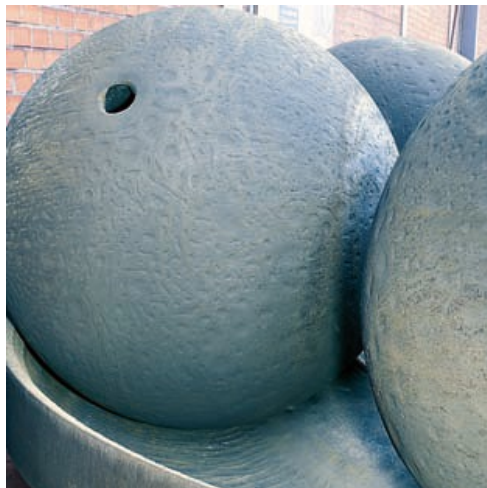
Grinding elements after 25,000hrs maintenance free operation.
