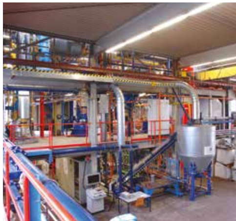
Technikum interior with grinding and pneumatic conveying systems.
