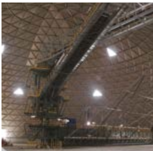
Circular blending bed for cement raw mix.
