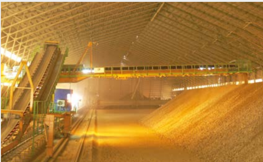
Stacker, mix of clay and limestone, 1200 tph, Algeria.
