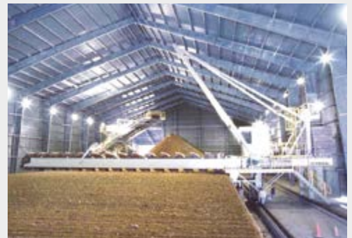
Bucket reclaimer, shale, 120 tph, USA.
