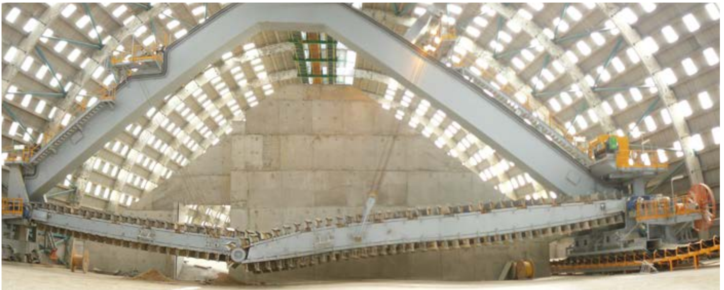
Portal reclaimer, fertilizer, 2200 tph, Morocco.
