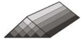
Windrow: Linear parallel superimposed layers
