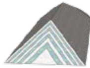
Chevron: Each layer discharged on top of preceding layer
