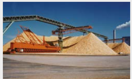
Circular stockyard for woodchips, 800 tph and 350 tph, Finland.
