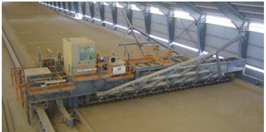
Longitudinal blending bed bridge reclaimer, limestone, 300 tph, Qatar.
