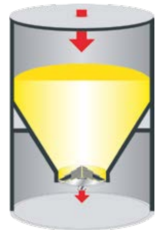
Cross section of CC silo.
