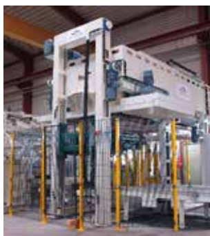
High Inlet Palletizers can process up to 5,000 bags/h.
