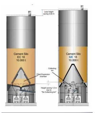
Figure 4. Technical comparison: construction and design of an EC silo (left) and ME silo (right).
