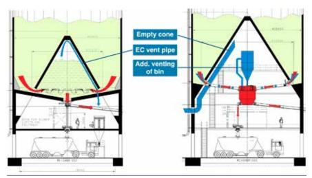
Figure 3. Technical comparison: operational behaviours of air and cement flow of an EC silo (left) and ME silo (right).
