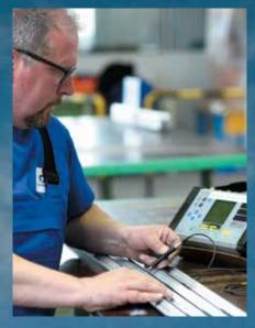
HFEC Surface Crack Testing.
